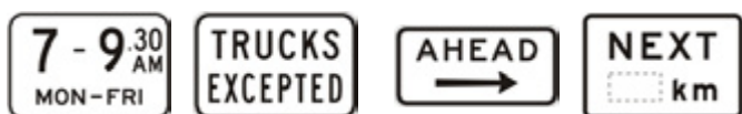
Time of operation sign, Trucks excepted sign, Ahead arrow sign, Distance sign
