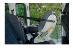
A regular rear facing restraint faces the back of the car, and stays in the car.
